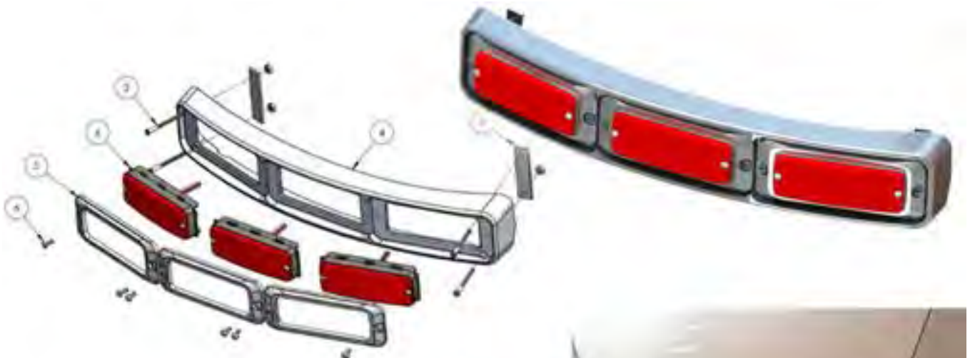
LH52711-1 & LH52712-1 Triple 500 Series Super LED TIR6, 2015 Ford Transit Cargo, Under-the-Headlight Housing Assembly
